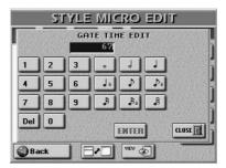
Here, you can either set the required length as a CPT value (J = 120CPT) or use the note fields to avoid lengthy calculations. Use the numeric pad to enter the desired duration. Drum parts usually use the Gate Time value "1" for all notes. Increasing it to "20", for example, has no audible effect on the sound durations. The maximum duration a note event can have is 99,999 clocks, which corresponds to roughly 208 bars.
